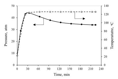
Fig. 1 Time dependences of pressure (•) and temperature (o) of urea synthesis by propylene carbonate ammonolysis.
