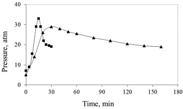
Fig. 3 Separate carrying out 1st (■) and 2nd (▲) stages of ammonolysis of propylene carbonate at 126 °C. Stage 1—NH<sub>3</sub>:PC = 2:1, PC—0.6 mol; stage 2—NH<sub>3</sub>:HPC = 2:1 (NH<sub>3</sub>/HPC ratio is calculated according to HPLC analysis of the products of stage 1).
